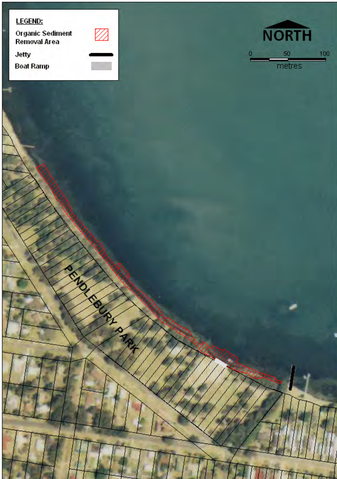
Figure 3.6 Bonnells Bay: Proposed Removal Works
